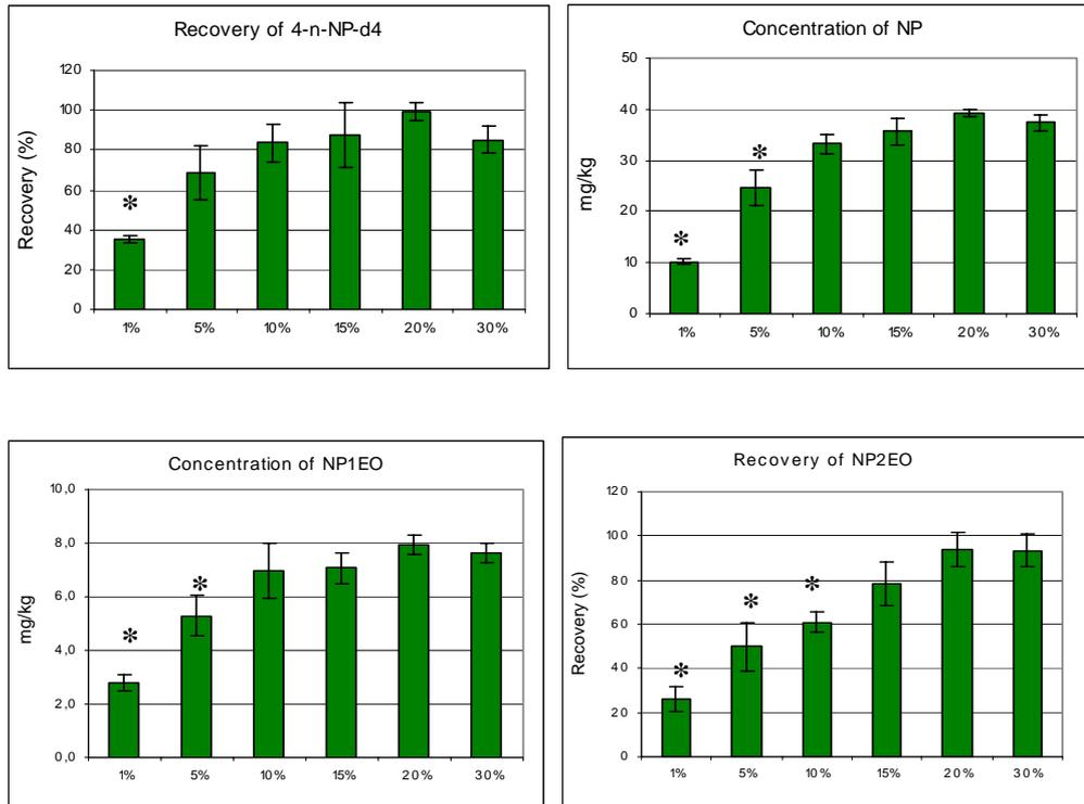
Figure 25. Concentration and recovery (%) of NP-D4, NP, NP1EO and NP2EO extracted from SL-E2. An asterisk above the column indicates significant ( $p = 0,05$ ) decrease in extraction efficiency ( $n = 3$ ).
