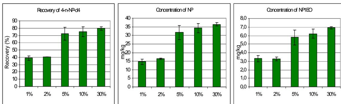
Figure 26.A. The recoveries of NP-D4, NP and NP1EO from sludge samples (SL-E2) with varying content of dry matter.
