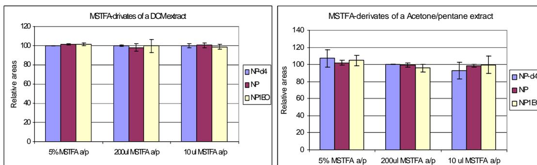
Figure 9. The responses (%) of NP-D4, NP and NP1EO in a) DCM-extract and b) Acetone/Pentane-extract submitted to different derivation procedure. The responses are calculated relative to the average response of the differently treated extracts. The error bars indicate standard deviation of the replicates (n = 2).
