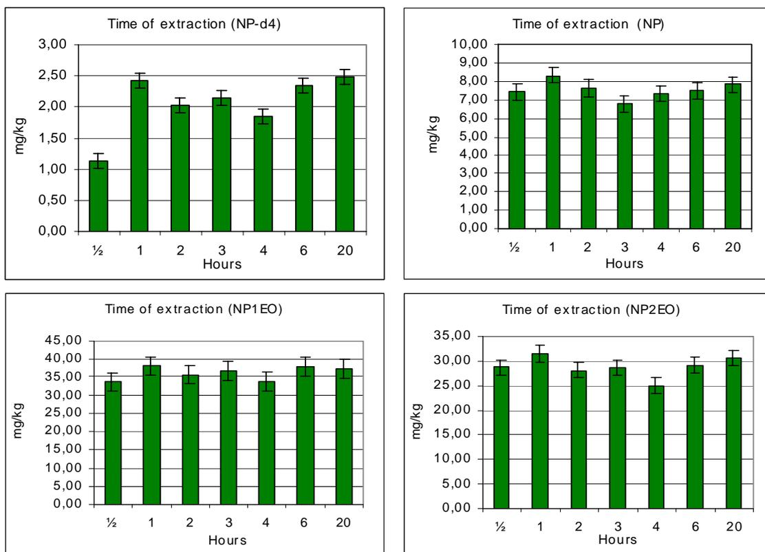
Figure 20. Concentration of NP-D4, NP, NP1EO and NP2EO extracted from freeze-dried sludge (SL-4). The quantification was based on phenanthrene-D10 as internal standard.
