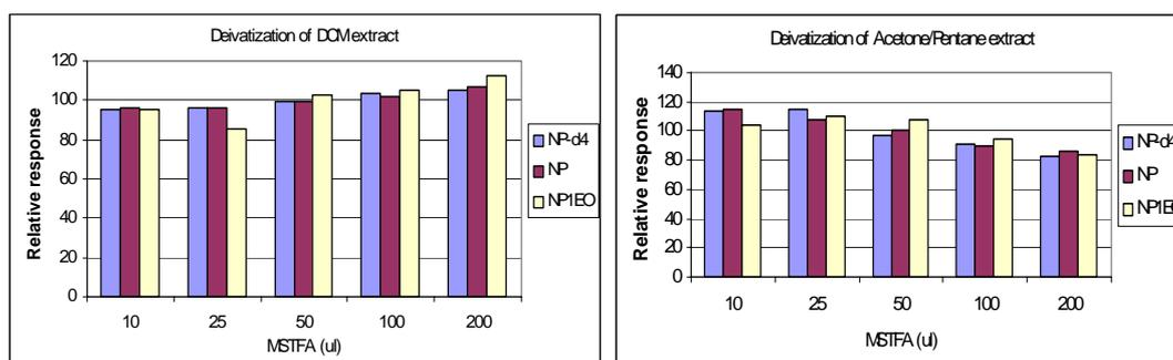
Figure 8. The responses (%) of NP-d4, NP and NP1EO treated with varying amounts of MSTFA (n = 1). The responses are calculated relative to the average response of the five treated extracts.
