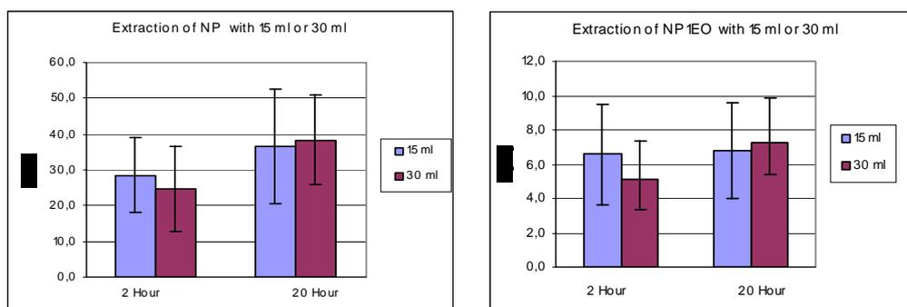
Figure 18. Extraction of a) NP and b) NP1EO from a sludge sample (SL-E2) conducted with 15 and 30 ml of solvent for 2 and 20 hours.
