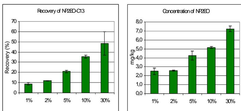
Figure 26.B. The recoveries of  $^{13}\text{C}$ - NP2EO and NP2EO from sludge samples (SL-E2) with varying content of dry matter.
