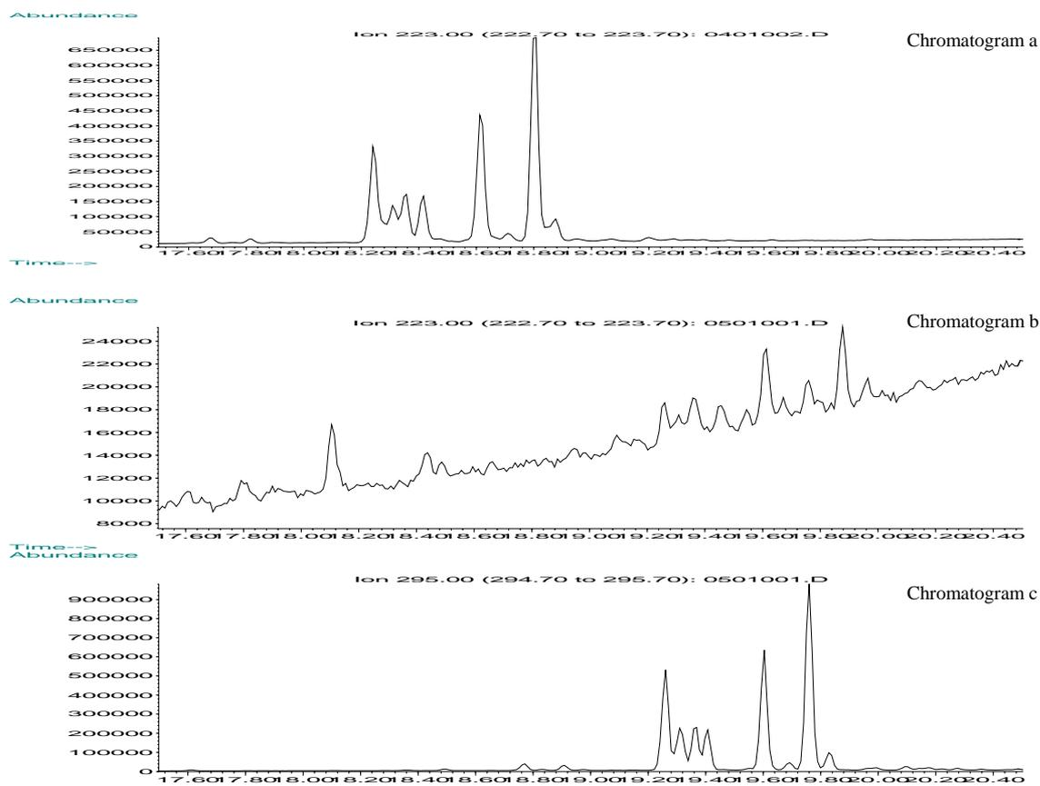
Figure 12: Chromatograms of a) a 20 mg/l un-derivatized NP2EO (ion 223), b) a 20 mg/l derivatized NP2EO (ion 223) and c) a 20 mg/l derivatized NP2EO (ion 295).
